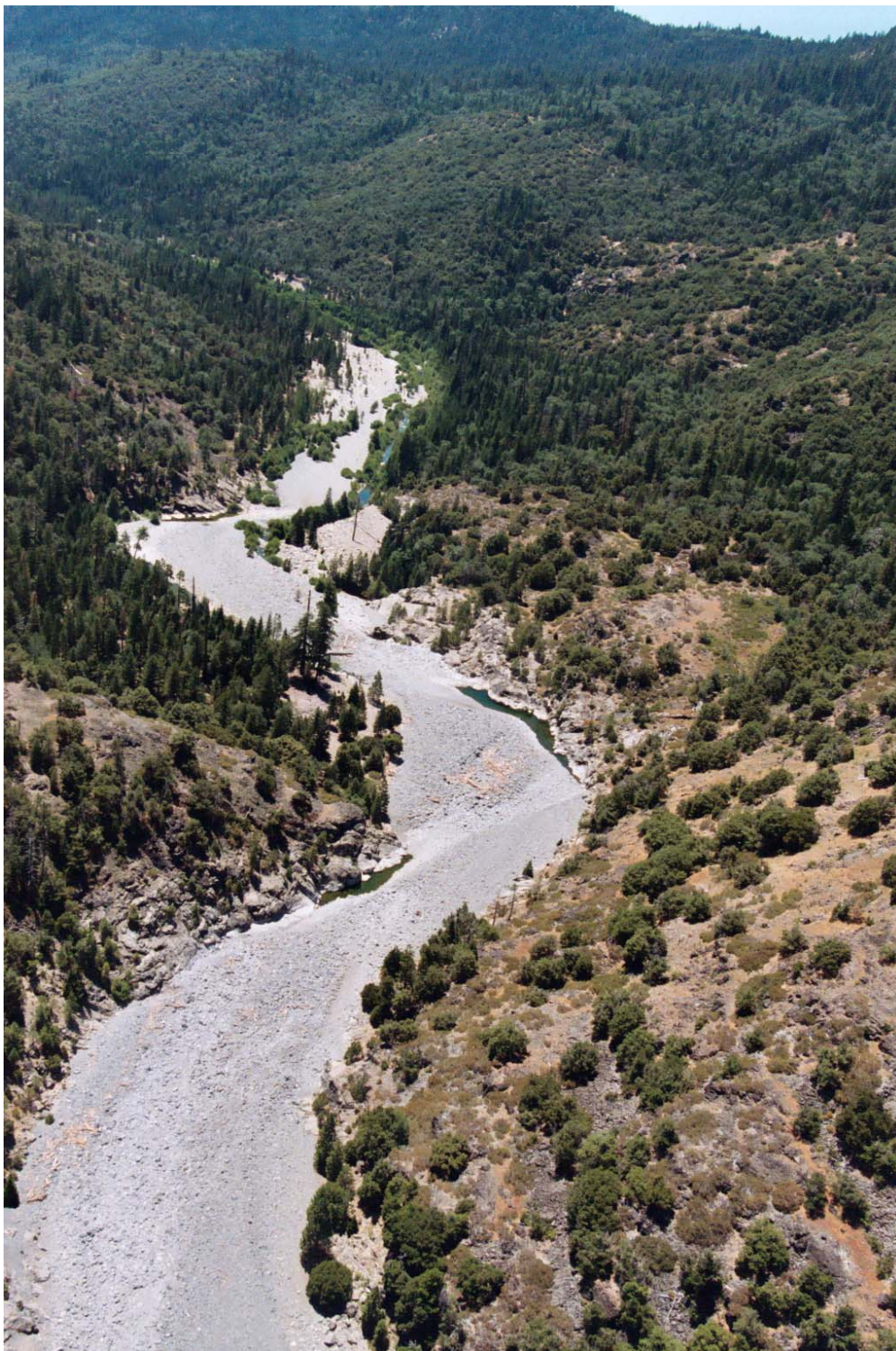
Photo F-8: Rubicon River, (RM 29) aggraded channel reach in debris field below Hell Hole Dam
