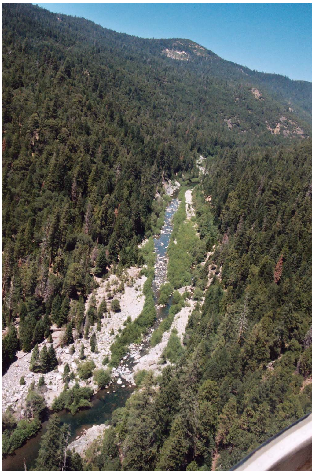
Photo F-7: Rubicon River (RM 26) Rosgen Level 1 B-channel type with a moderate entrenchment and width-depth ratio
