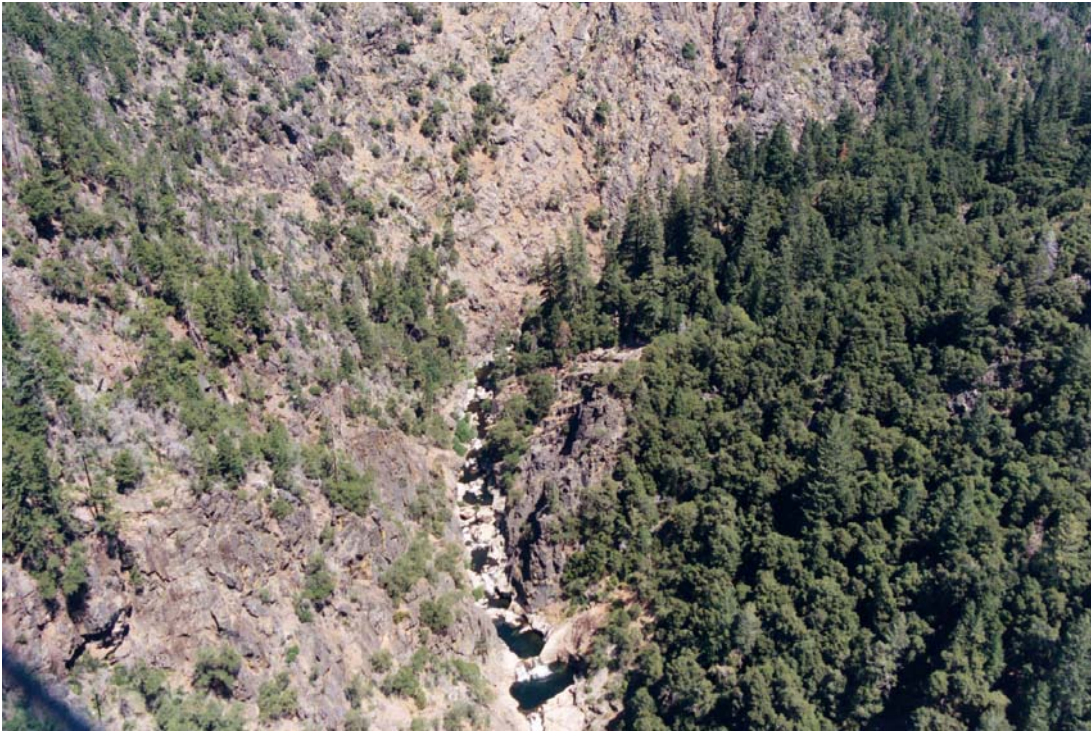
Photo F-5: Middle Fork American River (RM 40) Rosgen Level 1 A-channel type is highly entrenched steep with a low width-depth ratio
