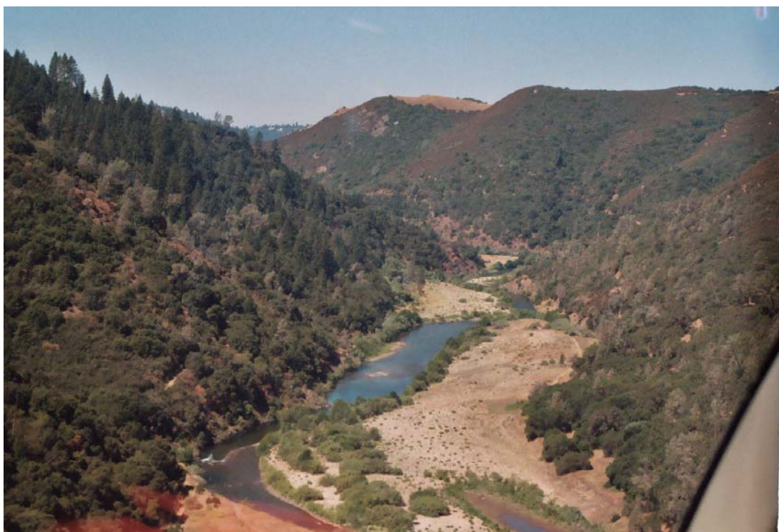
Photo F-4: Middle Fork American River (RM 13.0) Rosgen Level 1 F-channel type below Oxbow Reservoir
