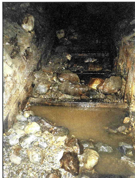
Tunnel sluice with mercury-contaminated sediments.
