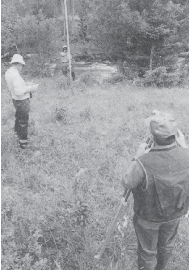
Figure 49. Good location for level setup.
