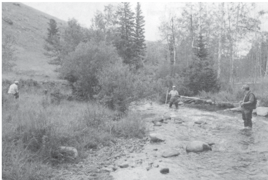
Figure 50. Measuring along the channel centerline and staking.
