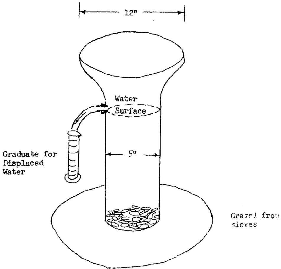
Figure 4. Device for volumetric measurement of gravel and sand fractions by displacement.
