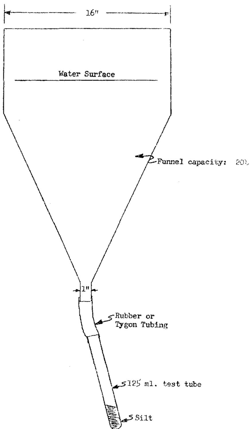
Figure 3. Settling funnel for determination of silt fraction.
