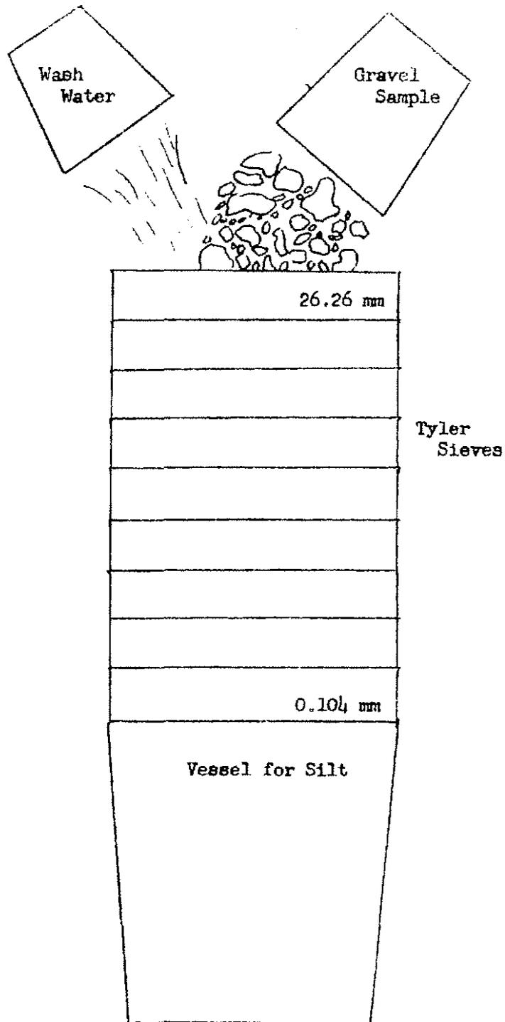
Figure 2. Arrangement of sieves and basin for separation of gravel sample.
