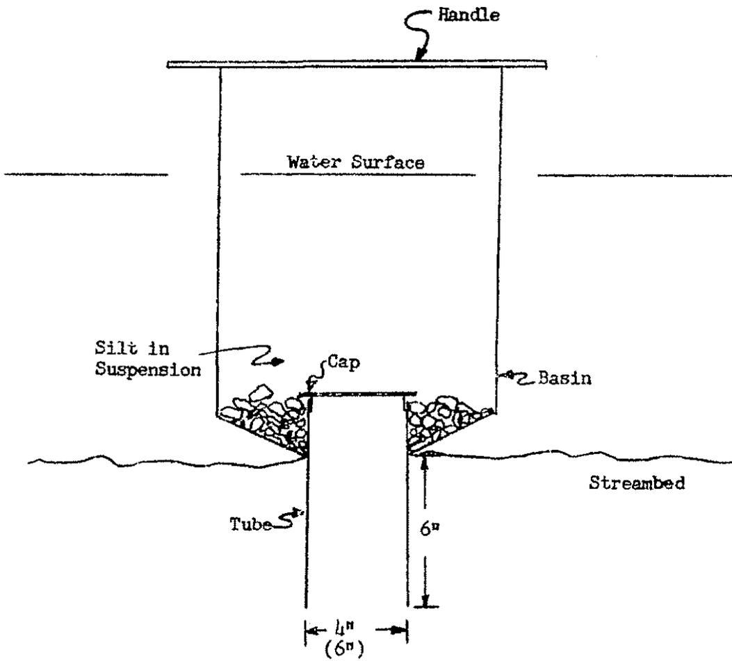
Figure 1. Gravel sampler.
