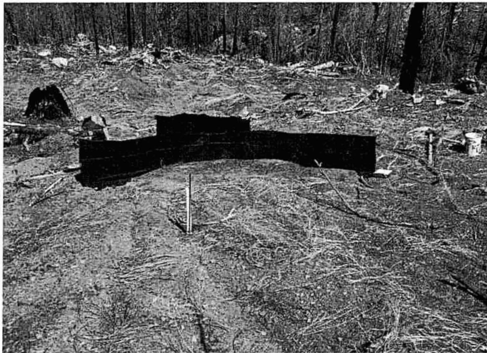
Figure 5. Typical sediment fence and crest gauge with a second fence installed to increase the sediment storage capacity. Picture taken in summer 2003 in a site that was tractor-logged in fall 2001.
